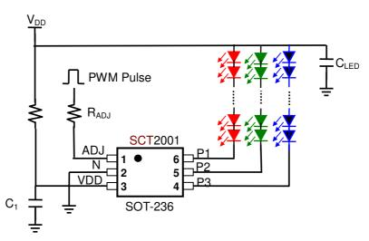
Maximizing the width and minimizing the length of VDD and GND trace improves efficiency and ground bouncing. Adding a capacitor  $C_{LED}$  greater than 10uF beside the LED is recommended.
