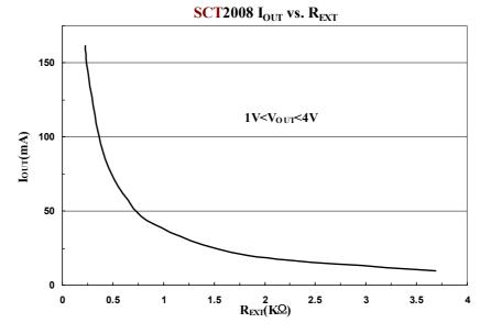
According to SCT2008' I-V curve, the output voltage should be larger than 1V to get 160 mA constant current. By applying proper output voltage, the SCT2008' output current set by an external resistor is approximate to:  $I_{OUT} = 60(630 / \text{REXT})$  (mA) (chip skew < ±6%). Thus the output current is set to be about 42mA at REXT = 900 $\Omega$ .
