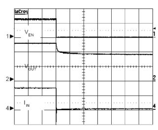
$\label{eq:VIN} \begin{array}{l} V_{\text{IN}} = 12 \text{V}, \ L = 10 \mu\text{H}, \ C_{\text{COMP}} = 0.22 \mu\text{F} \\ \text{CH1: } V_{\text{EN}}, \ 10 \text{V/div}, \ \text{DC} \\ \text{CH2: } V_{\text{OUT}}, \ 10 \text{V/div}, \ \text{DC} \\ \text{CH4: } I_{\text{IN}}, \ 500 \text{mA/div}, \ \text{DC} \\ \text{TIME: } 10 \text{ms/div} \end{array}$
