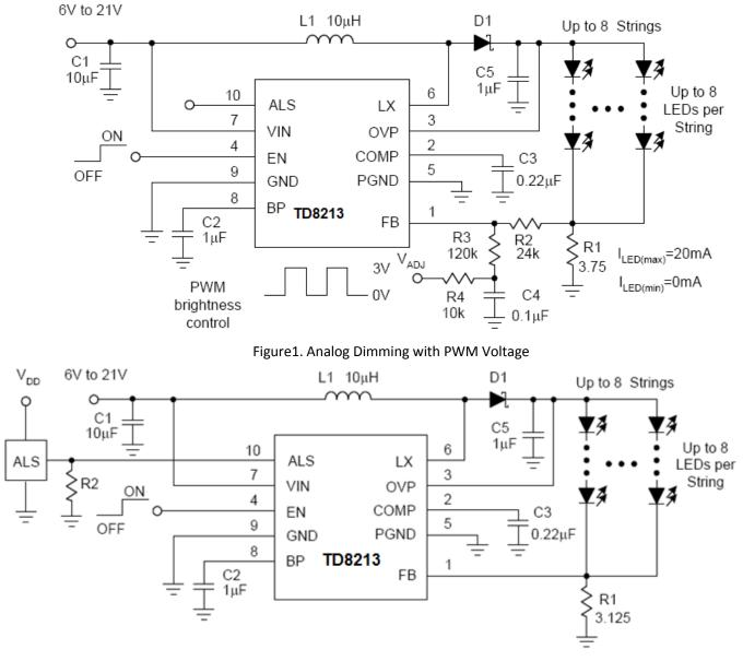
Figure2. Analog Dimming with External ALS Voltage
