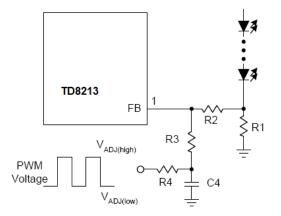
Figure 3. Dimming with the PWM Voltage
