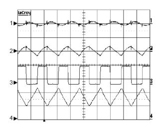
$\begin{array}{l} {\sf V}_{\sf IN}{=}12{\sf V},\,{\sf L}{=}10\mu{\sf H},\,{\sf C}_{\sf COMP}{=}160{\sf mA}\\ {\sf CH1:}\,{\sf V}_{\sf IN},\,50{\sf mV}/{\sf div},\,{\sf AC}\\ {\sf CH2:}\,{\sf V}_{\sf OUT},\,200{\sf mV}/{\sf div},\,{\sf AC}\\ {\sf CH3:}\,{\sf V}_{\sf LX},\,20{\sf V}/{\sf div},\,{\sf DC}\\ {\sf CH4:}\,{\sf I}_{\sf L},\,200{\sf mA}/{\sf div},\,{\sf DC}\\ {\sf TIME:}\,0.5\mu{\sf s}/{\sf div}\\ \end{array}$
