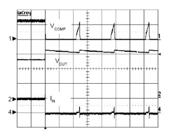
Output is open CH1: V<sub>COMP</sub>, 0.5V/div, DC CH2: V<sub>OUT</sub>, 10V/div, DC CH4: I<sub>IN</sub>, 100mA/div, DC TIME: 10ms/div
